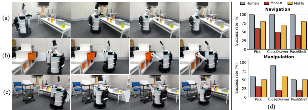
Figure 9: Real-world deployment on a Toyota HSR. Representative successful MoFlo rollouts for (a) PICK, (b) CLOSEDRAWER, and (c) PUSH SHELF, each shown as a left-to-right filmstrip from the predicted base pose through manipulation. (d) Navigation and manipulation success rate for each task and method (Human, Mobi- \pi , and MoFlo; out of 10 trials per task).
